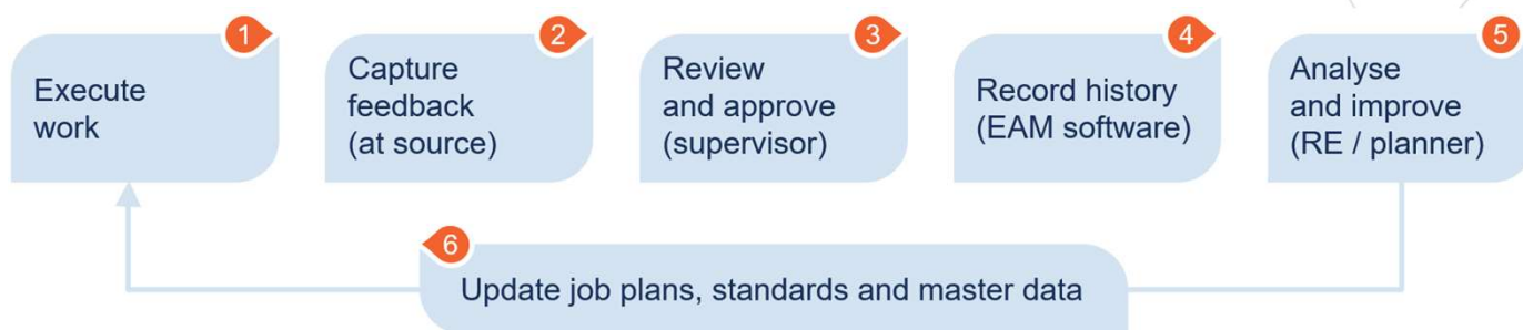
Figure 2: A closed feedback loop turns maintenance history into learning and better planning
